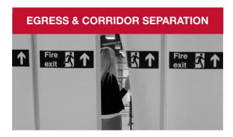
Protect escape routes for mass evacuation. The evacU8 smoke curtain allows egress through a compartment that contains smoke. It offers the capability to split deployment to encourage safe evacuation psychology where assemblies cross potential escape routes.
